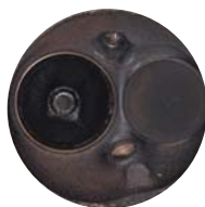
Cylinder head before P.i. treatment.
